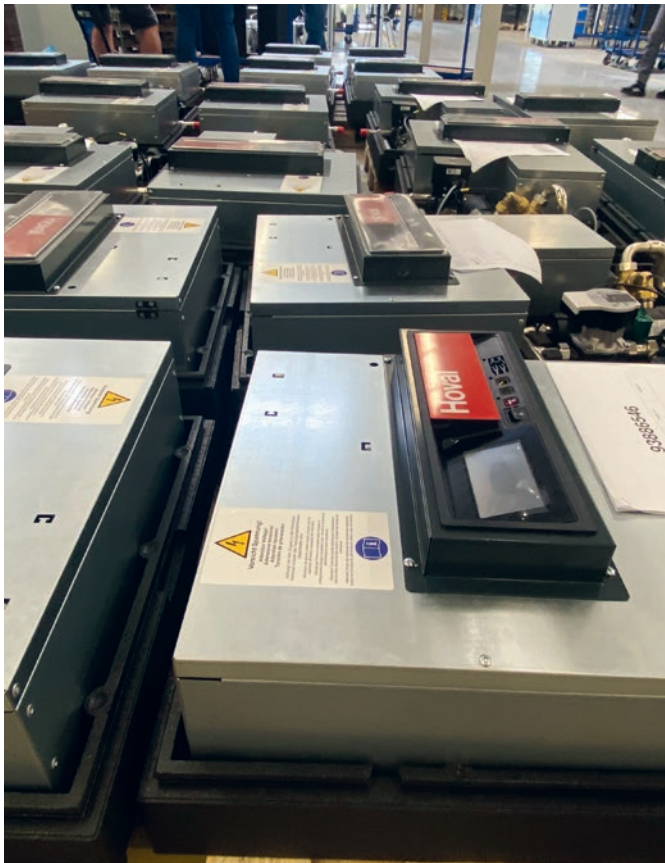
Heating modules of the Belaria® heat pump before shipping to Marchtrenk.
