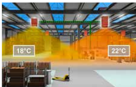
Decentralised units enable different temperature zones to be created.
